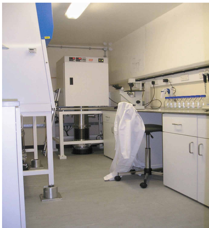
Fig. 3. The tissue culture facility established on the THz beamline. One THz line can be seen entering through the floor of the laboratory and into the bottom of the CO 2 incubator in the centre of the photograph. A second THz line enters through the bottom of the microbiological safety cabinet on the left. The THz output from the beamline can be switched between these lines for the radiation of live human tissue
