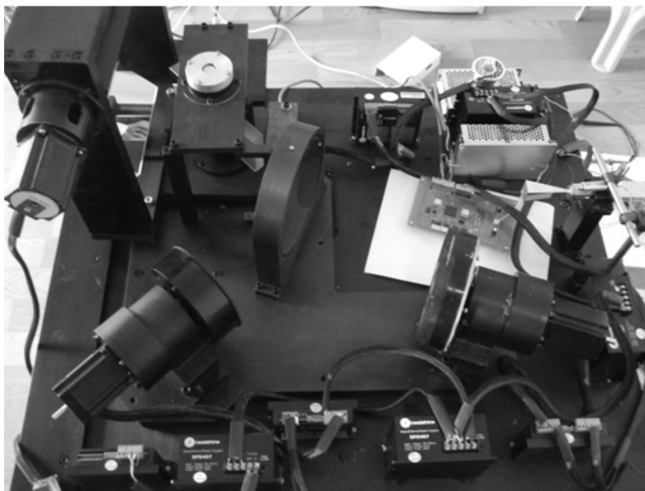
Fig. 6. Photo of the opto-mechanical THz scanner
